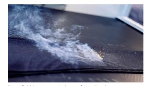
Laser finishing process being performed on jeans.
